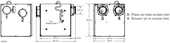
NOTE: ALL UNITS PORTS WERE CREATED TO BE CONNECTED TO DUCTS HAVING A MINIMUM OF 4" DIAMETER, BUT IF NEED BE, THEY CAN BE CONNECTED TO BIGGER SIZED DUCTS BY USING AN APPROPRIATE TRANSITION (E.G.: 4" DIAMETER TO 5" DIAMETER TRANSITION).
